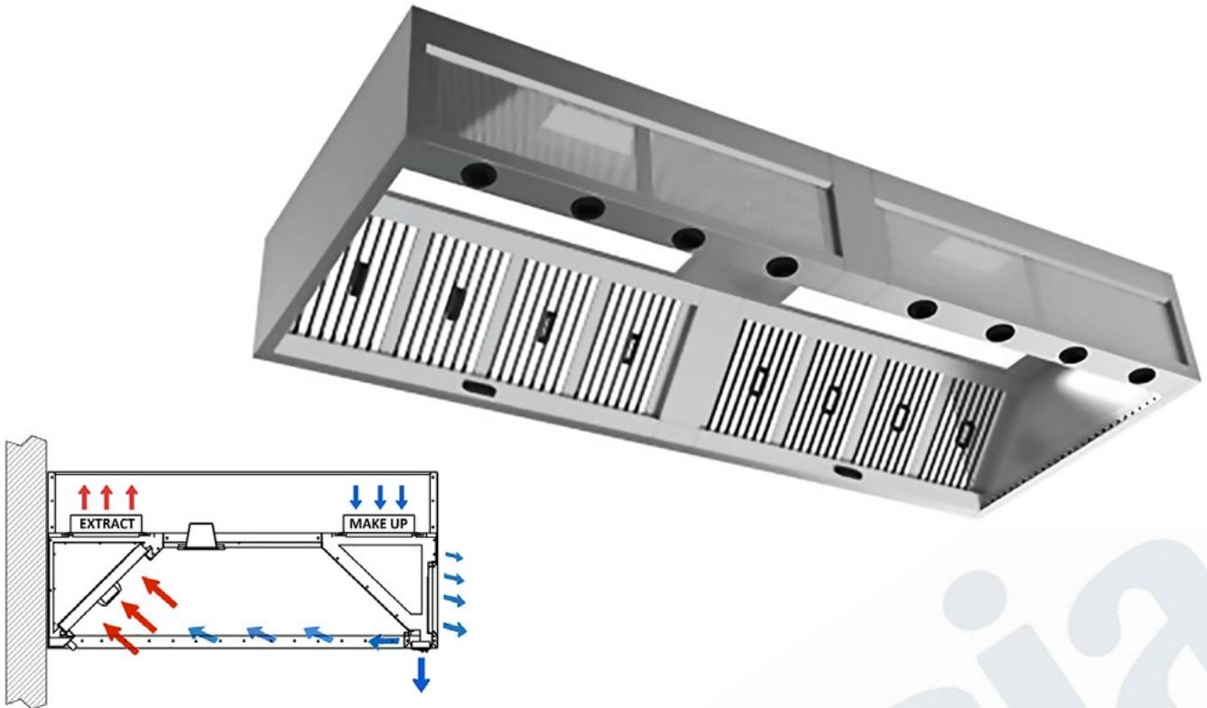
Britannia Capturestream 'CS3' Canopies offer total control over make-up air by providing diffused air to the front, spot cooling and the patented 'Capturestream' of air across the canopy from the front and two sides for superior performance through intelligent design and world-class baffle filter technology, all contributing to lower exhaust air rates.
