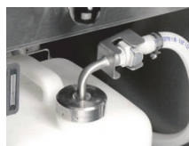
Oil replenished automatically from JIB for multi-well (left) or reservoir for 1-well (right)
