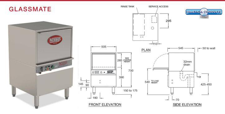
The Glassmate is a tough and reliable glasswasher manufactured to operate under the most demanding conditions. Fit with an optional cooling cycle designed to minimise the turnaround of glassware, this machine will prove to be reliable and dependable in the busiest of work environments. 10 amp version available.
